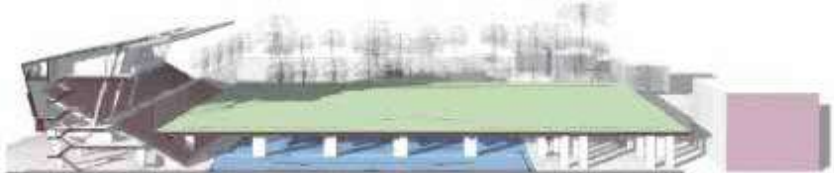
Plans for Apia Leichhardt's new stadium at Lambert Park with training fields on ground level and the main synthetic-grass pitch to be built on mega-concrete pylons.
